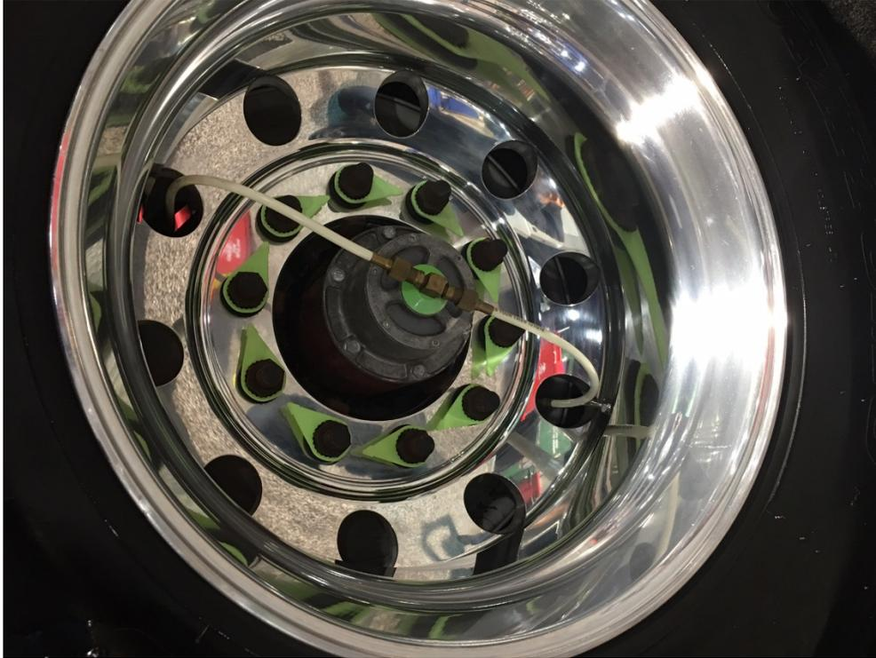
BENLEE now sells automatic tire inflation systems that after a puncture or leak has been detected they will keep most tires inflated until they can be serviced. Importantly, these systems can be retrofitted on existing trailers.
